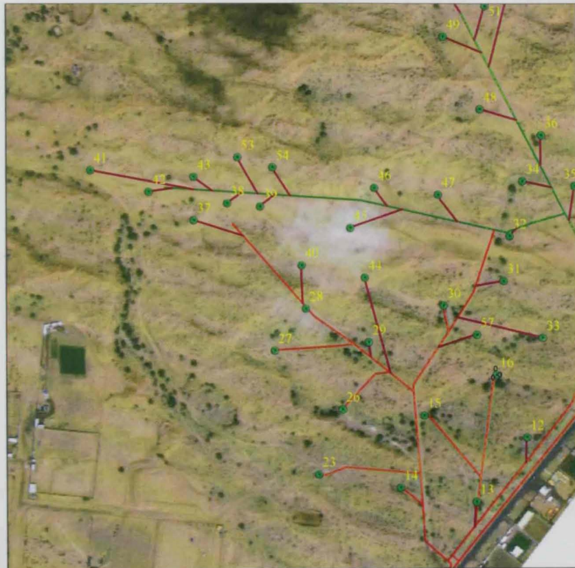
Figure 4.3. Water wells connected through pipe network
